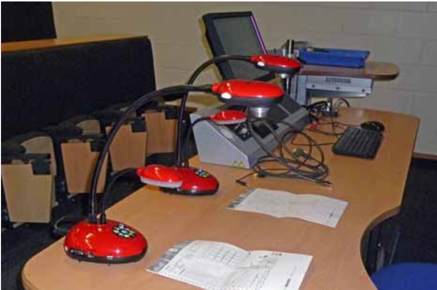
Clever coding by the Bath AV team enables images from the twin DC192 units in the larger lecture theatres to be displayed side by side by a single projector:
