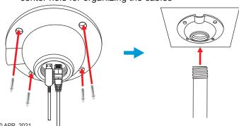
3.2 Loosen the screws on both sides to remove the camera locking platform. After sticking the anti-slip mats, use spring washers and screws one by one to mount the platform on the camera base.
